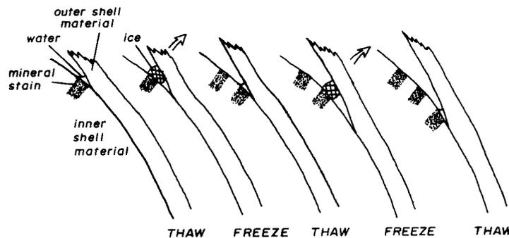
Figure 4: hypothetical freeze/thaw mechanism for incremental staining of inner shell material (see text)
