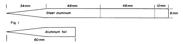
of the folded aluminum strip as in Figure 3 and strike sharply with the tack hammer (you may want to practice this step on some other scraps of aluminum; I managed to get it right the first time). This causes the tip of the forceps to have a small groove and to be slightly splayed out, which facilitates the holding of round, slippery specimens and keeps them from squirting out sideways.
