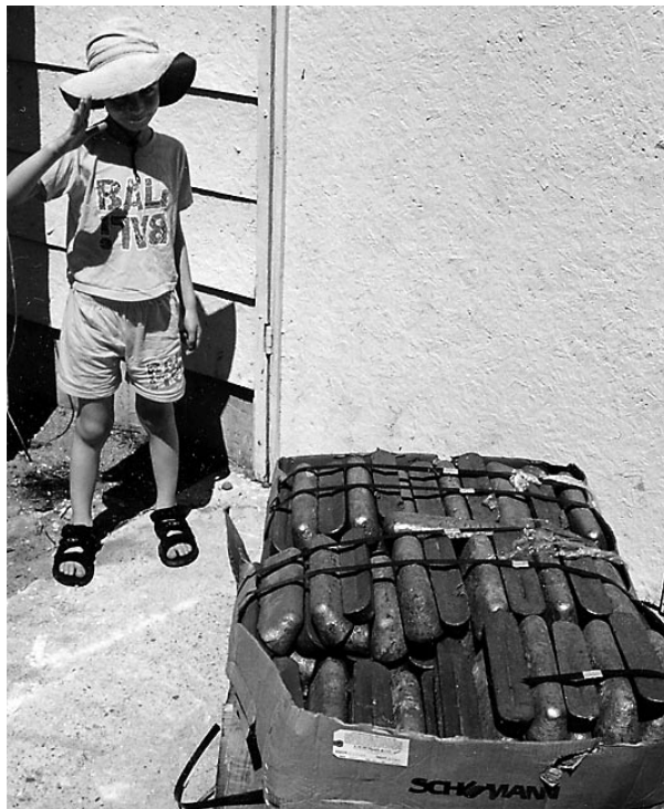
Bronze ingots: raw material for the art castings. Next stop is the smelter oven.
