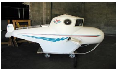
Figure 4. The minisub Free Diver is similar to this 1990 SportSub II seen on a wheeled cart. Manufacturer: International VentureCraft Corporation, Burnaby, BC (Website: www.ivccorp.com ). Dimensions: L 3.05 m, W 1.83 m, H 1.40 m. Weight (dry): 565 kg (1250 lb.); Payload capacity (in water): 180 kg (400 lb.); Occupant capacity: 2; Maximum diving depth: 40 m (130 ft); Top speed (underwater): 5 knots (9.25 km/h or 6 mph); Hull construction: fiberglass; Powered by 2 continuously variable thrusters at port and starboard, 75 pounds thrust each. Photograph from company's website.
