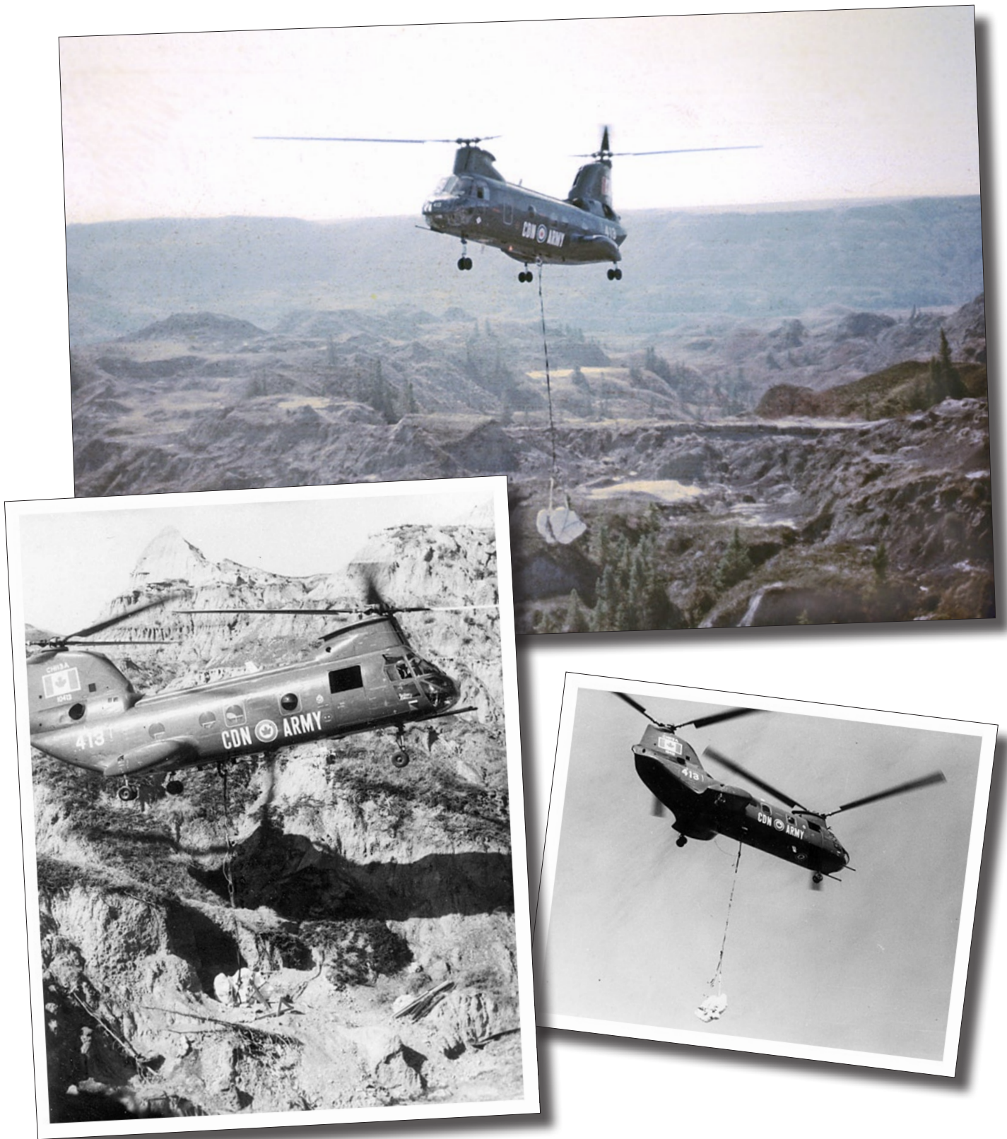
Figure 15. Lower left: The CH-113A moments after first lifting the block. The machine is dark olive green overall with red/white Canadian flag and roundel, and white lettering. The helicopter's shadow shows how close it was to the ground. Top and lower right: Free of the confines of the surrounding badlands, the block makes its short journey up to prairie level where it will be lowered into a waiting truck. The lower right image also appears in Anonymous, 1968d. Photographs courtesy of Philip J. Currie (top), via Alan Lindoe, formerly of the University of Alberta; and Jane Danis and the Department of National Defense (lower).
