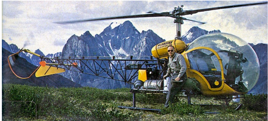
Figure 4. An early model Bell 47. This was the type most extensively used by the GSC in Canada during the 1950s and proved ideal for rugged fieldwork. Landing gear were either skids or pontoon floats. It may be recognizable to some readers as the Korean War medical evacuation helicopters used in the 1972–1983 hit television series M*A*S*H *. The Bell 47 was produced from 1946 to 1974. Image from Callison, 1983.
