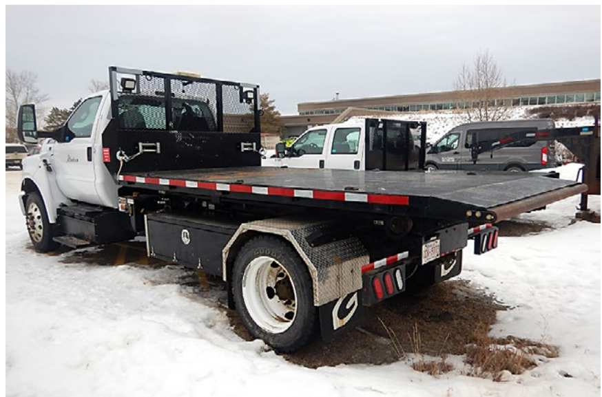
Figure 7. The RTMP’s 2019 Ford F650 Super Duty truck with SL145 swap loader deck. The flat deck measures 3.79 m long and 2.19 m wide. A slightly downward angled rear end of the deck creates a longer platform (4.13 m). The tilting and removable deck stands 1.32 m above ground. The deck has two strong winches, each rated at 6.8 t. The hook lift on the truck can lift 6.3 t. Photo by the author.
